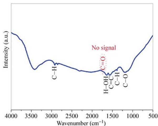
**Figure 4** FTIR spectrum of the GNRs. No obvious signal characteristic of a carboxylic group can be observed at  $1730\text{ cm}^{-1}$  (indicated by the dotted ring), indicating considerable deoxygenation of GNRs
