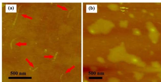
**Figure 5** (a) AFM image of short GNRs (indicated by red arrows) produced by sonication treatment for a duration of more than 10 h. (b) AFM image of small graphene pieces obtained from GSs with a high percentage of oxygen-containing groups (C/O:  $\sim 6.0$ )
