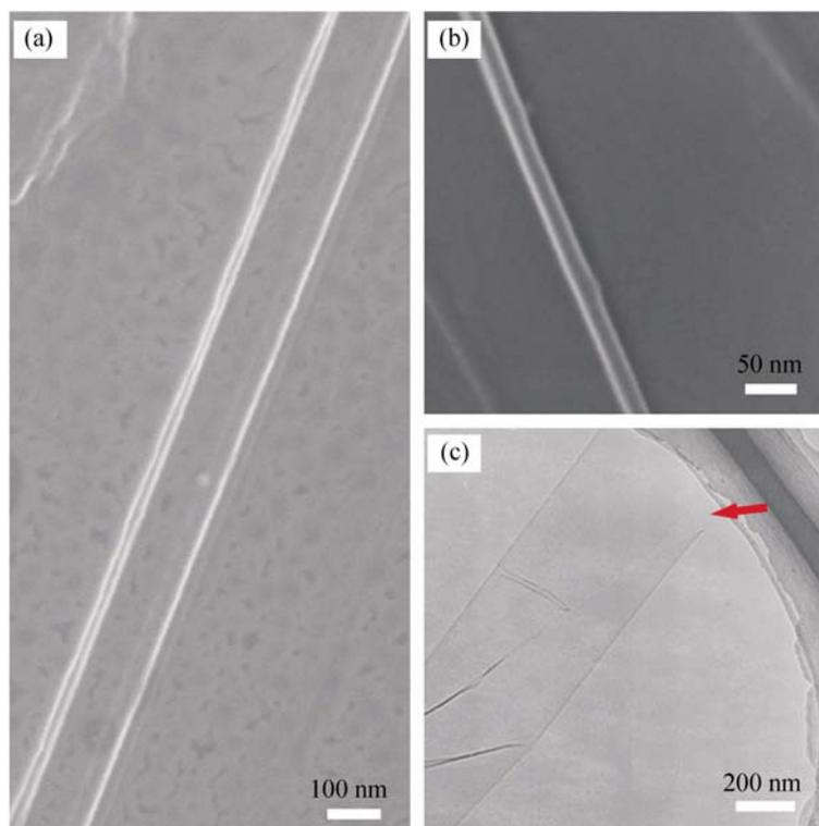
**Figure 6** (a) SEM image of three long parallel line faults (white lines) on the GO surface, with separations of several nanometers to tens of nanometers. (b) Two parallel line defects on the GS surface with a separation of ~25 nm. (c) TEM image of the as-prepared GS, showing evidence of cutting GSs along the line fault (indicated by a red arrow)
