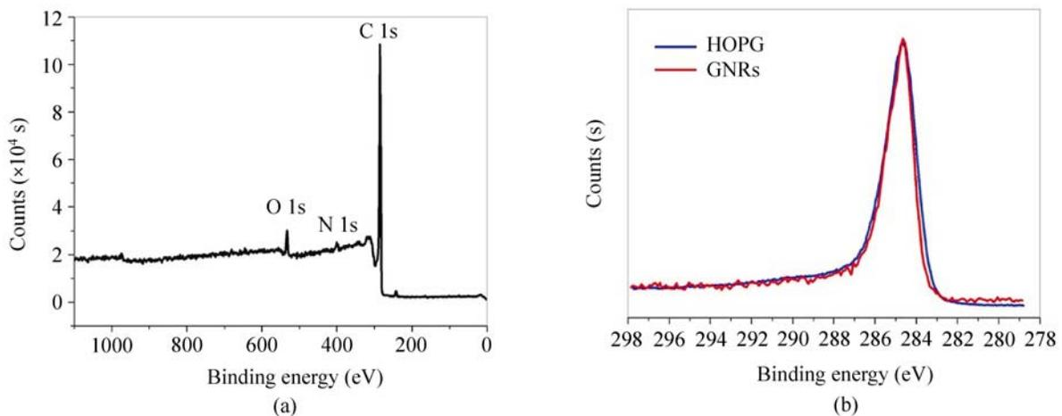
**Figure 3** (a) XPS of GNRs recorded between 0 and 1100 eV. (b) The intensity normalized C 1s XPS of GNRs (red line) and pristine HOPG (blue line). The similarity of the spectral features shown in (b) indicates that the GNRs were considerably deoxygenated
