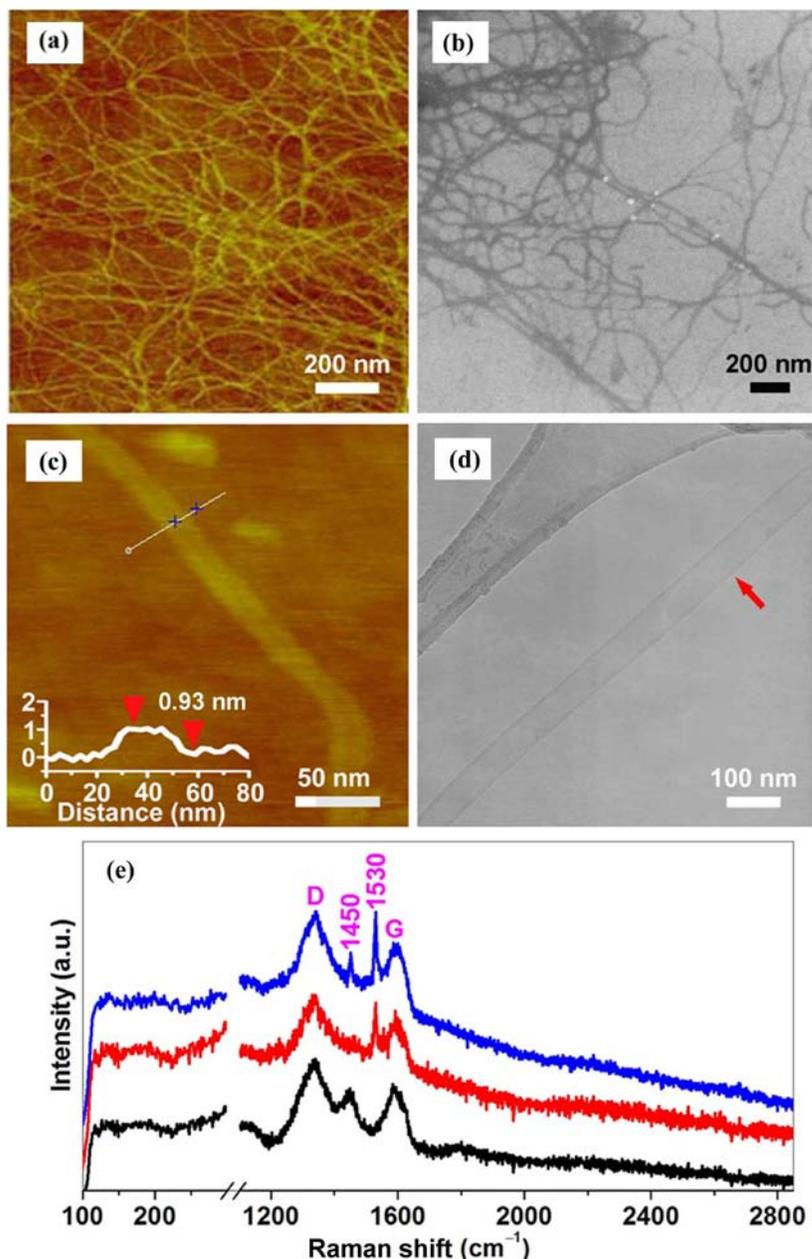
**Figure 1** (a) AFM and (b) SEM images of the GNRs spin-coated from the GNR supernatant on a Si substrate capped with 300-nm-thick  $\text{SiO}_2$ . (c) AFM image of an individual GNR. Inset: the height profile reveals that the measured GNR has a height of ~0.93 nm and width of ~20 nm. (d) TEM image of a GNR with a width of ~60 nm (indicated by a red arrow). (e) Typical Raman spectra of the as-prepared GNRs on a Si substrate capped with 300 nm thick  $\text{SiO}_2$
