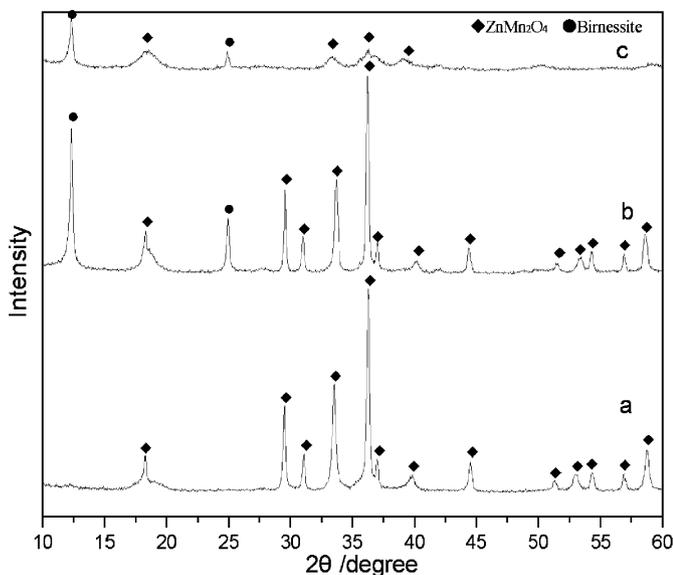
Fig. 6. XRD patterns of the samples obtained hydrothermally at 170 °C for 48 h at the Zn/Mn ratio of 0.6 with different zinc sources: (a)  $\text{Zn}(\text{CH}_3\text{COO})_2 \cdot 2\text{H}_2\text{O}$ , (b)  $\text{ZnSO}_4 \cdot 7\text{H}_2\text{O}$  and (c)  $\text{ZnCl}_2$ .
