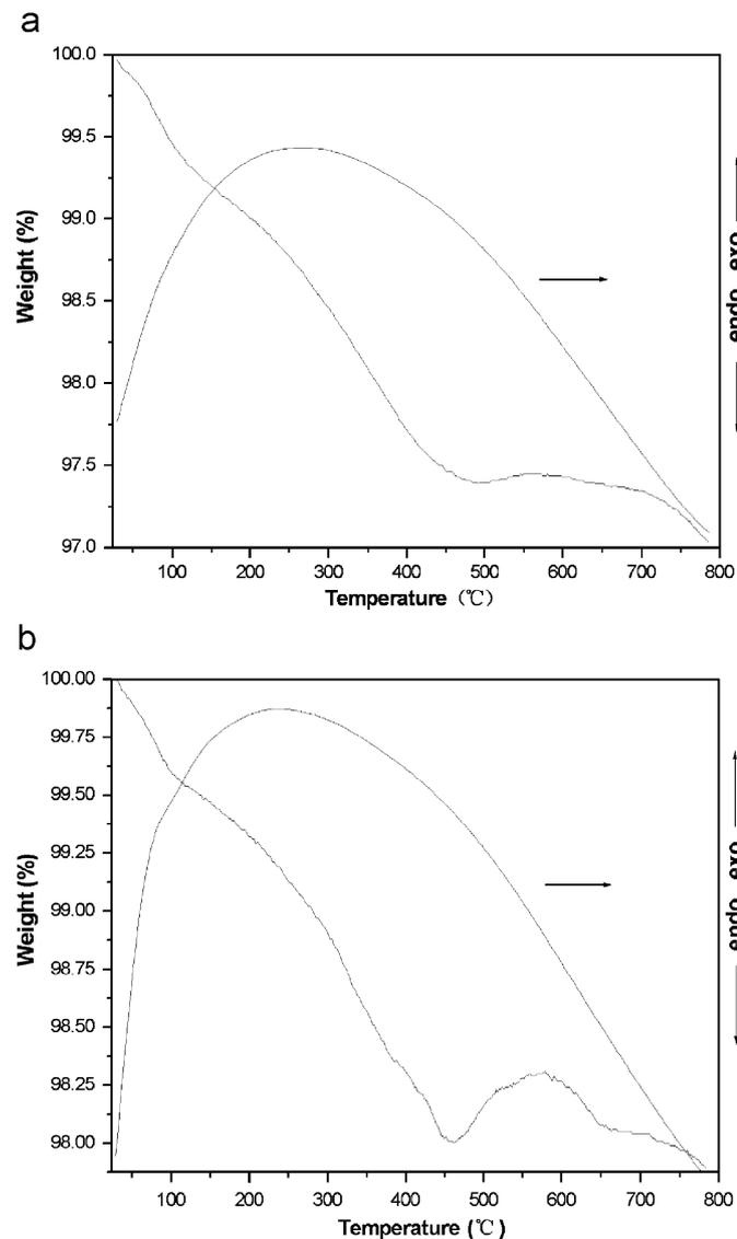
Fig. 10. TG curve of the sample obtained hydrothermally at 170 °C for 48 h at the Zn/Mn ratio of (a) 0.55 and (b) 0.6, respectively.
