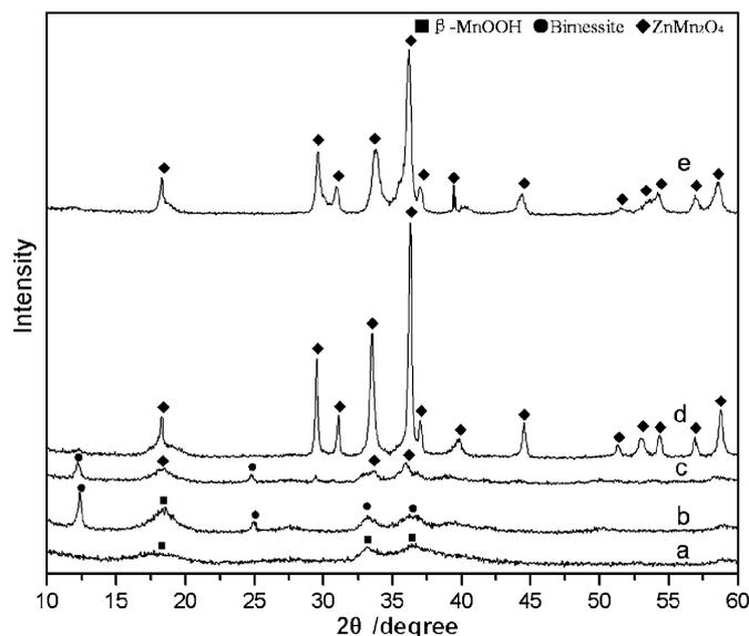
Fig. 5. XRD patterns of the samples obtained hydrothermally at the Zn/Mn ratio of 0.6 at 170 °C for the reaction time of (a) 0 h, (b) 12 h, (c) 24 h, (d) 48 h and (e) 72 h, respectively.
