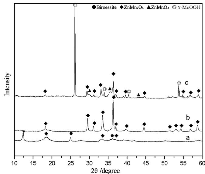
Fig. 3. XRD patterns of the samples obtained hydrothermally at (a) 150 °C, (b) 170 °C and (c) 190 °C for 48 h at the Zn/Mn ratio of 0.6.
