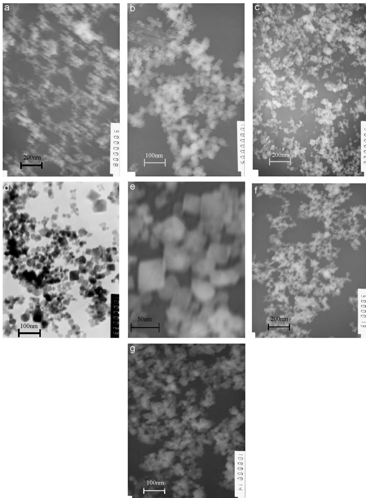
Fig. 2. Low and high-magnification TEM images of the samples obtained hydrothermally at 170 °C with the Zn/Mn ratios of 0.55 (a, b), 0.6 (c, d, e) and 0.65 (f, g), respectively.
