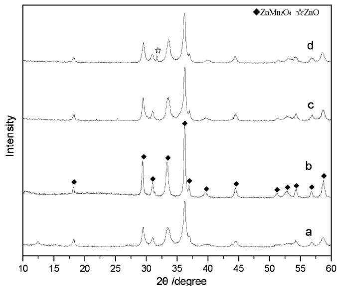
Fig. 8. XRD patterns of the samples obtained hydrothermally at 170 °C for 72 h at the Zn/Mn ratio of (a) 0.5, (b) 0.6, (c) 0.8 and (d) 1.0, respectively.
