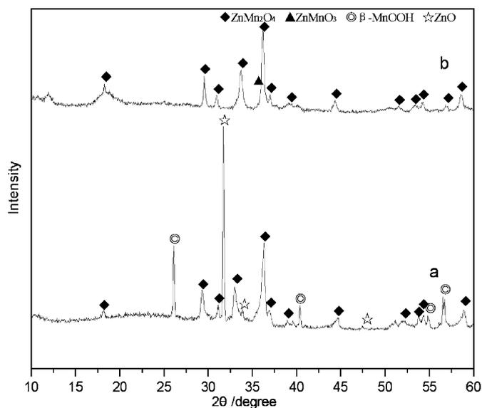
Fig. 7. XRD patterns of the samples obtained hydrothermally at 170 °C for 48 h from (a) 5 ml NaOH and 0.92 ml  $\text{H}_2\text{O}_2$  and (b) 6 ml NaOH and 1.2 ml  $\text{H}_2\text{O}_2$  at the Zn/Mn ratio of 0.6.
