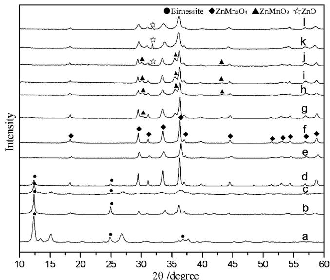
Fig. 1. XRD patterns of the samples obtained hydrothermally at 170 °C for 48 h at different Zn/Mn ratios of (a) 0, (b) 0.2, (c) 0.4, (d) 0.5, (e) 0.55, (f) 0.6, (g) 0.65, (h) 0.7, (i) 0.75, (j) 0.8, (k) 0.9 and (l) 1.0.
