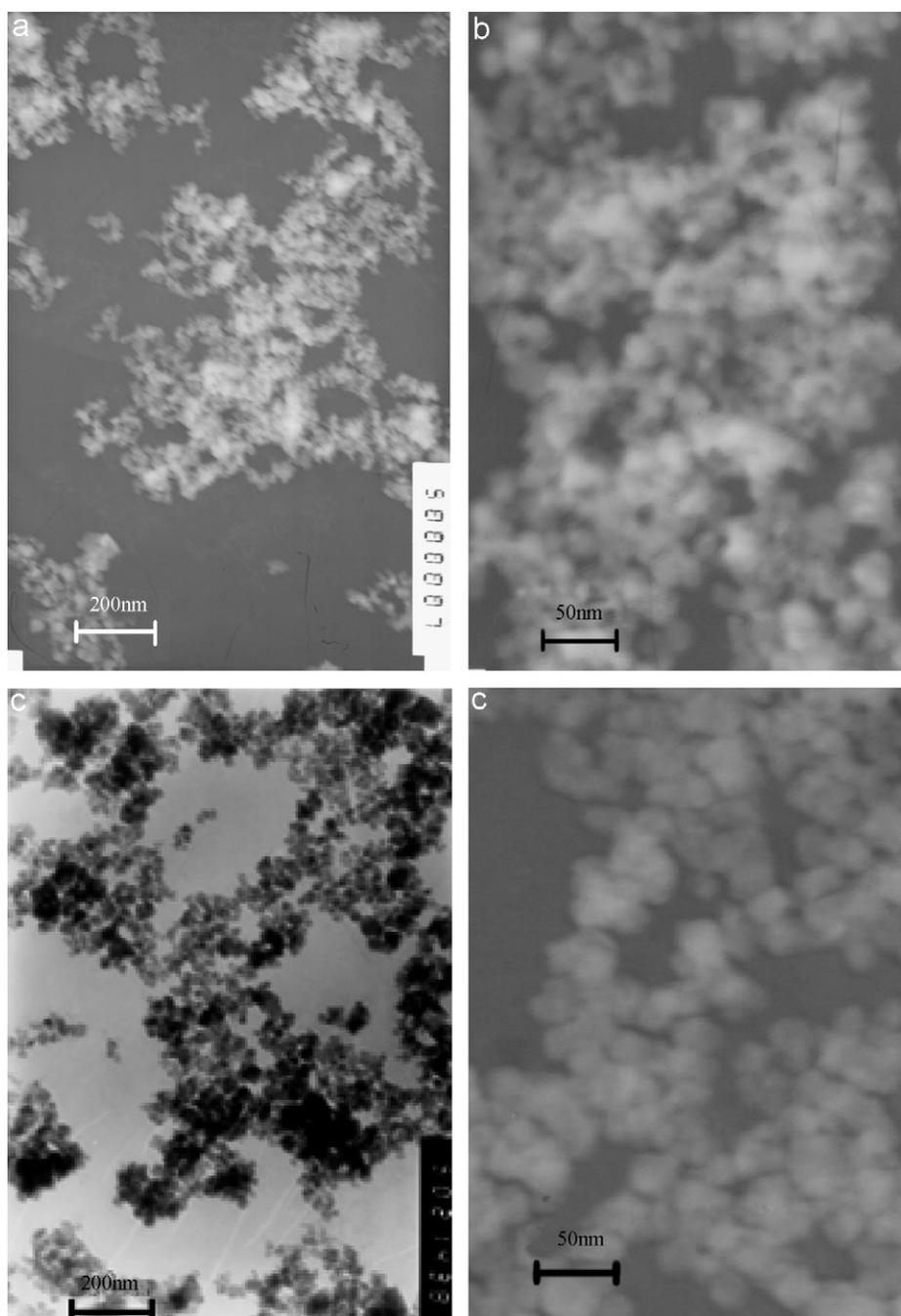
Fig. 9. Low and high-magnification TEM images of the samples obtained hydrothermally at  $170^\circ\text{C}$  for 118 h at the Zn/Mn ratio of 0.55 (a, b) and 0.65 (c, d), respectively.
