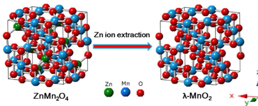
Scheme 1. Representation of the unit cell of \text{ZnMn}_2\text{O}_4 spinel prepared by ultralow-temperature hydrothermal synthesis and \lambda\text{-MnO}_2 defect spinel obtained from \text{ZnMn}_2\text{O}_4 by acid leaching.
