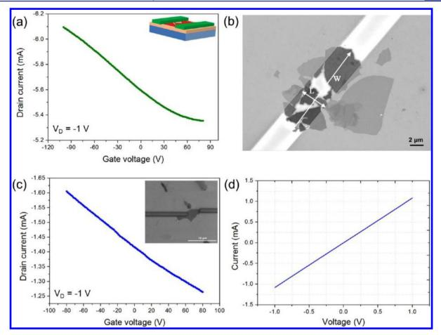
**Figure 6.** (a) Transfer curve for a FET device based on an EG thin film. (b) SEM image of the fabricated device showing thin EG flakes between the Au electrodes. Channel length and width are indicated by arrows. (c) Transfer curve of a FET device based on single-layer EG (inset is the SEM image of the fabricated device). (d) Current–voltage (I-V) curve of an isolated single-layer EG flake.
