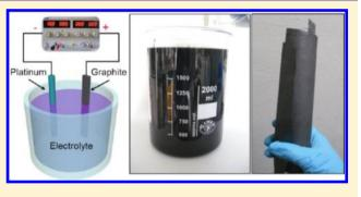
solid-state flexible supercapacitors manufactured on the basis of such graphene films deliver a high area capacitance of 11.3 mF  $cm^{-2}$  and an excellent rate capability of 5000 mV s<sup>-1</sup>. The described electrochemical exfoliation shows great promise for the industrial-scale synthesis of high-quality graphene for numerous advanced applications.
