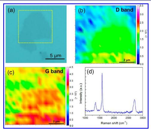
Figure 4. (a) Optical microscopic image of an EG flake. Scale bar 5  $\mu$ m. (b, c) Raman intensity maps for D and G peaks, respectively. (d) Representative Raman spectra. The Raman excitation laser wavelength is 532 nm.
