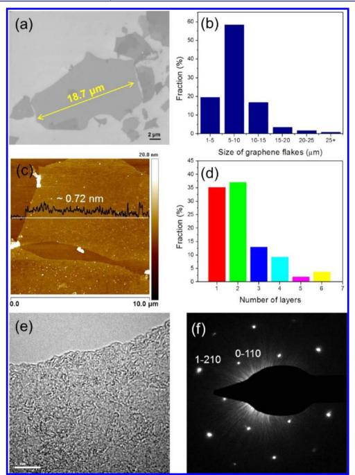
Figure 3. (a) SEM image of EG. (b) Statistical flake size analysis of graphene sheets by SEM., (c) AFM image of EG on silicon substrate. (d) Statistical thickness analysis of EG by AFM. (e) HRTEM of single-layer graphene. (f) SAED pattern of EG.
