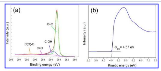
Figure 5. (a) XPS C 1s spectra of EG. (b) The secondary electron cutoff of EG measured from ultraviolet photoemission spectra.
