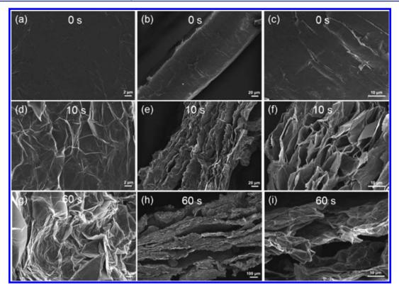
Figure 2. SEM images of (a,d,g) surface and (b,e,h) edge morphology of the graphite foil after applying a bias voltage of +10 V for 0, 10, and 60 s in aqueous  $(NH4)_2SO_4$  electrolyte solution, respectively. (c,f,i) Magnified images of panels b, e, and h, respectively.
