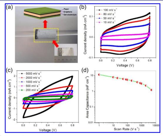
**Figure 8.** (a) Photographs of supercapacitor based on EG ink-coated paper, where the device is rolled around a glass rod. Inset shows a photograph of the device prior to rolling. (b and c) Cyclic voltammetry curves of EG paper-based supercapacitor (loading 0.6 mg cm<sup>-2</sup>) at scan rates from 10 to 100 mV s<sup>-1</sup> and 200 to 5000 mV s<sup>-1</sup>, respectively. (d) Evolution of area capacitance versus scan rate.
