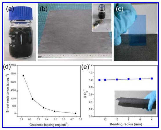
Figure 7. (a) Photograph of EG in DMF (10 mg mL<sup>-1</sup>) used as an ink. (b) Commercial A4-size paper coated with EG using a paintbrush (inset). (c) Film adhesion test with cellophane tape. (d) Relationship between the resistances of the paper with graphene loading. (e) Changes in sheet resistance after bending the conductive paper into different radii.
