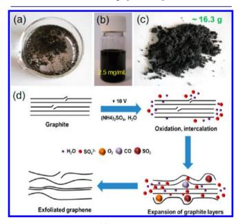
Figure 1. Photograph of (a) graphite flakes after electrochemical exfoliation, (b) dispersed EG in DMF solution (concentration ~2.5 mg mL<sup>-1</sup>), (c) EG powders on a bulk scale (~16.3 g). (d) Schematic illustration of the mechanism of electrochemical exfoliation.
